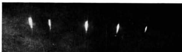
Fig. 2. The first layer line of the 2H polytype found on the opposite face to the 12H polytype (Fig. 1) (before annealing).
