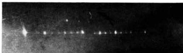
Fig. 1. The first layer line of lead iodide 12H polytype (before annealing).
